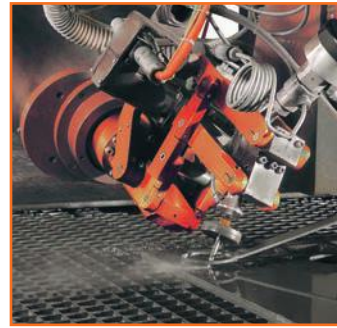
3D (5-axis) cutting head (optional)
