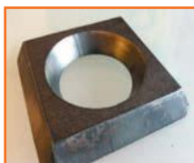
Bevel in 12 mm (0.47") St37 steel
