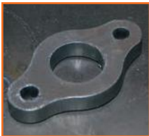
High Precision drilling in 4 mm (0.16") St37 steel
